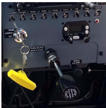
Figure 5: Central panel (yellow lever: Tow cable release, middle lever: Throttle, right lever: Cockpit heating)
